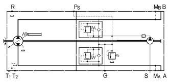
Assignment Direction of rotation - Control - Direction of through put flow
