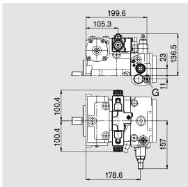
Control valve, fixed setting and hydraulic inch valve mounted, DA4/DA8
