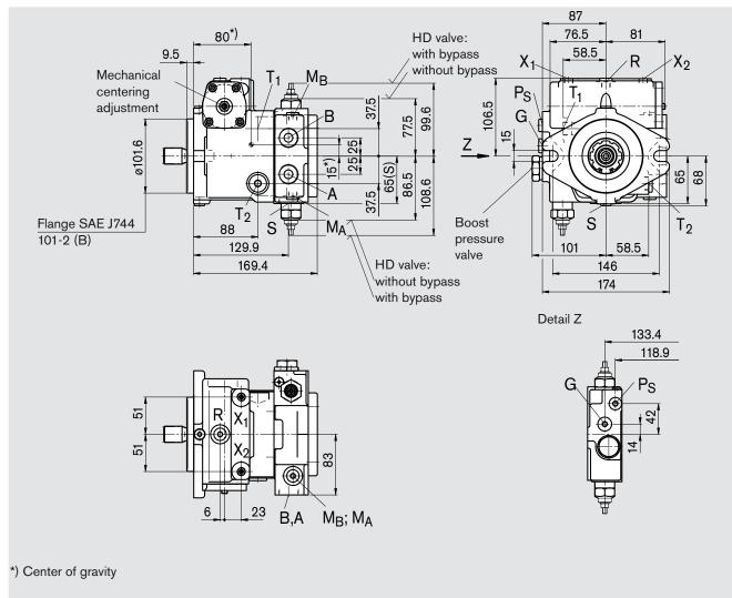
Before finalizing your design, please request a binding installation drawing. Dimensions in mm.
