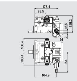
Control valve, fixed setting and hydraulic inch valve mounted, DA4/DA8
