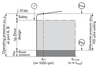
Example: boost pressure 20 bar; operating pressure 290 bar
