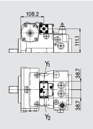
Electric two-position control with switching solenoid, EZ
