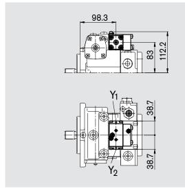
Electric two-position control with switching solenoid, EZ
