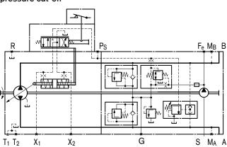
Version with DA control valve, neutral position switch and pressure cut-off
