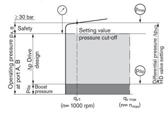
Example: boost pressure 20 bar; operating pressure 290 bar
