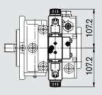
Mechanical pivot control, spring neutral position centering, MDN
