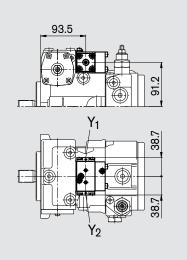
Electric two-position control with switching solenoid, EZ
