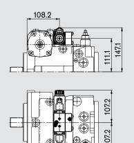
Hydraulic control, speed related, DA Control valve, fixed setting, DA2
